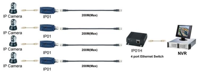
Caution: IP01H unit with BNC male terminator at channel 2, 3, 4. Do not remove the terminator if you do not use these channels. Otherwise, it will cause this Switch not working.
