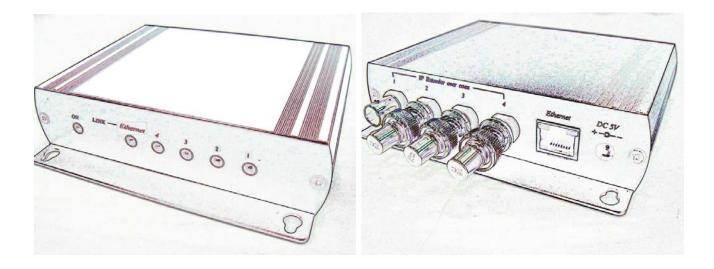
IPO1H 4 port Ethernet Switch is special design and built in 4 pieces IPO1 (IP extender over coax) with BNC interface to send and extender TCP/IP signal over coaxial cable. Used in set with IPO1 at IP camera side or any TCP/IP equipment, to send the IP signal up to 200 meters over your existing coax cable. 4 BNC port based on 10Mbps transmission speed, 1 port RJ45 to your NVR/computer based on 10/100Base-T.
